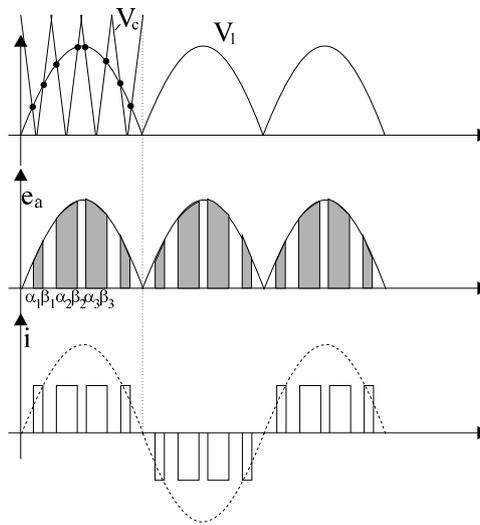
Figure 5.19. Single-phase full converter with PWM control
