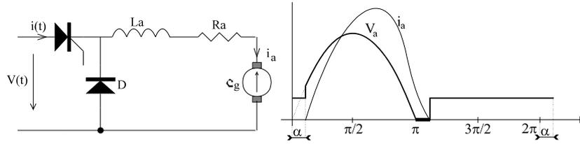
Figure 5.1. A DC brush motor supplied through a thyristor
