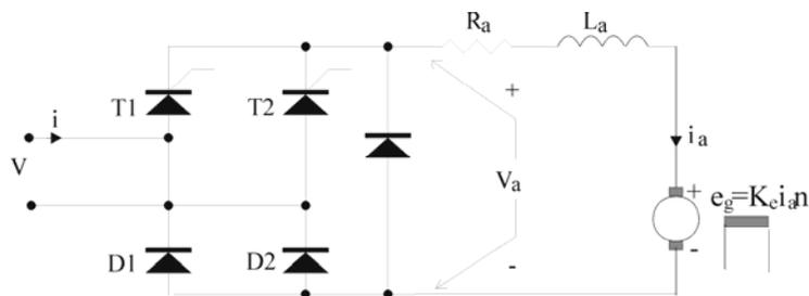
Figure 5.18. DC series motor supplied through a single-phase semiconverter
