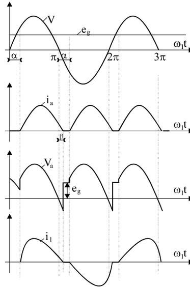
Figure 5.4. D.c brush motor supplied from a full converter – discontinuous current mode
