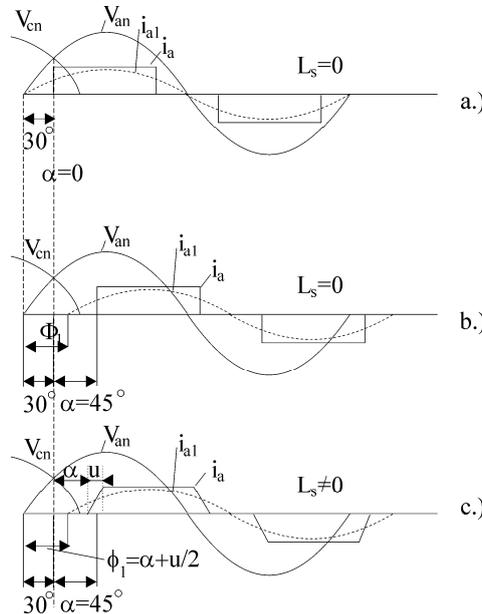
Figure 5.8. AC source currents in a three-phase full converter and constant motor current: a.) for  $\alpha = 0$ ,  $L_s = 0$ ; b.) for  $\alpha = 45^\circ$ ,  $L_s = 0$ ; c.) for  $\alpha = 45^\circ$ ,  $L_s = 1\text{mH}$
