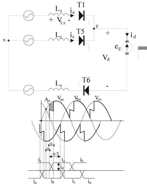
Figure 5.7. The current commutation in the presence of AC source side inductances  $L_s$ .
