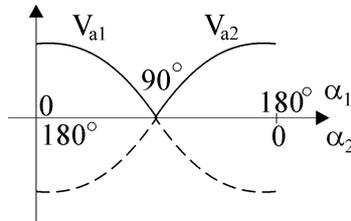
Figure 5.11. Ideal dual converter voltages
