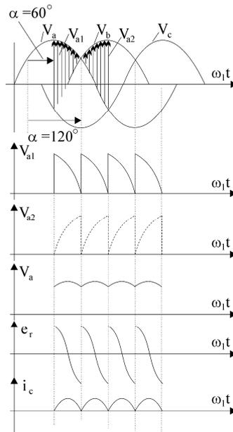
Figure 5.12. The real dual converter
