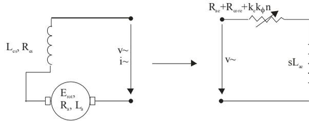
Figure 5.13. The equivalent scheme of universal motor
