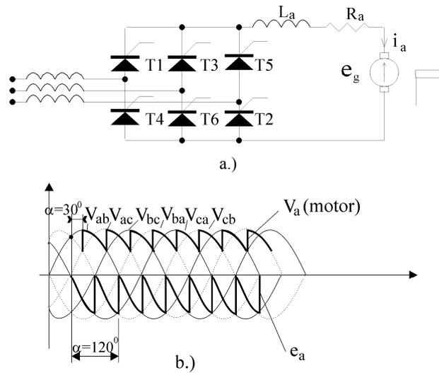
Figure 5.6. DC brush motor fed from a three-phase full converter
