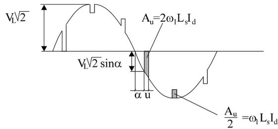
Figure 5.9. AC source-line voltage notches due to  $L_s$  (commutation)
