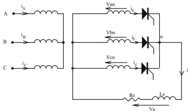
Figure 5.17. Three-phase rectifier with controlled null
