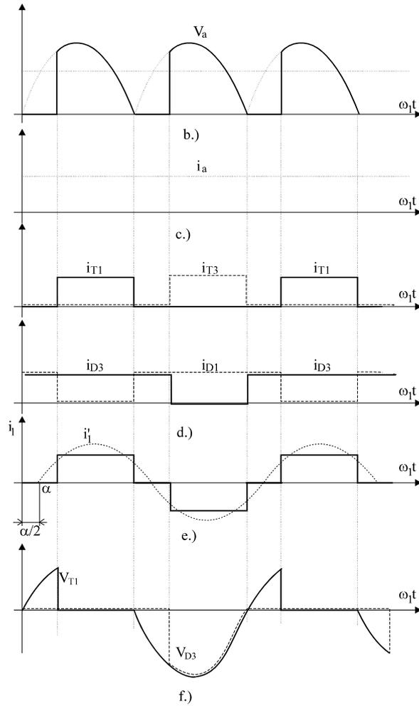
Figure 5.2. DC brush motor supplied through a single-phase semiconverter (with large inductance  $L_a$ )
