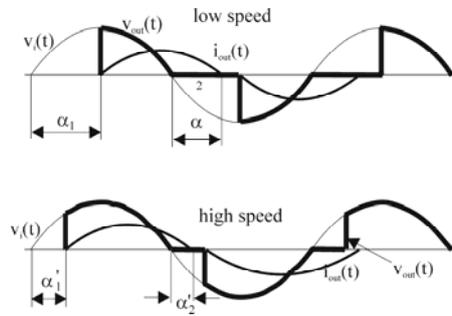
Figure 5.15. Output voltage and current waveforms at low and high speed
