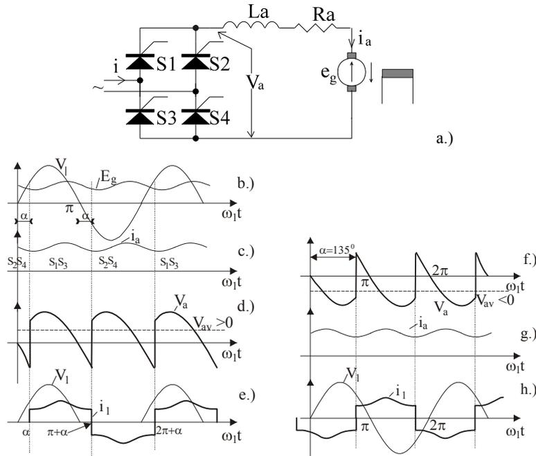
Figure 5.3. The DC brush motor fed through a single-phase full converter:
