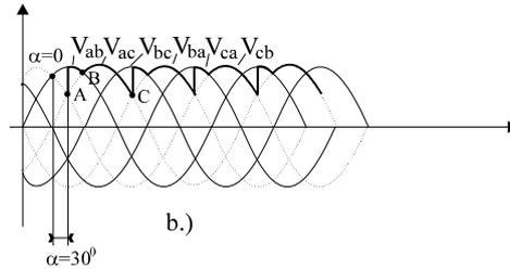
Figure 5.5. DC brush motor supplied through a three-phase semiconverter
