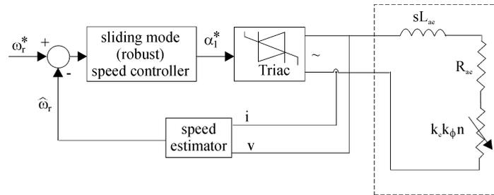
Figure 5.16. Generic control system for universal motors
