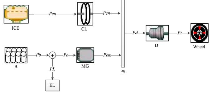
Fig. 2. The parallel PHEV topology
