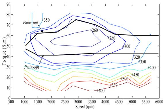
Fig. 3. SI41 engine specific fuel consumption map in the CD mode (g/kWh)
