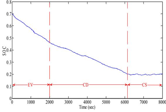
Fig. 1. PHEV operation modes
