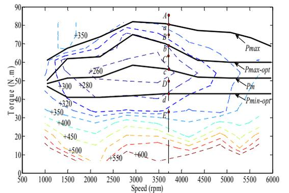
Fig. 5. The SI41 engine operation area in the CS mode.
