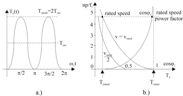
Figure 4.14. AC brush series motor steady state characteristics:
