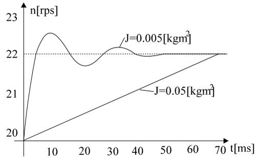
Figure 4.10. Speed responses to a step voltage increase from 110V to 120V at constant load torque
