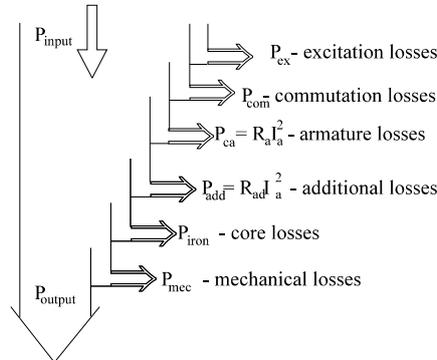
Figure 4.4. Loss breakdown in DC brush motors
