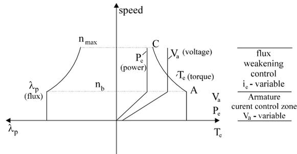
Figure 4.7. Speed/torque, power, voltage envelopes for constant current
