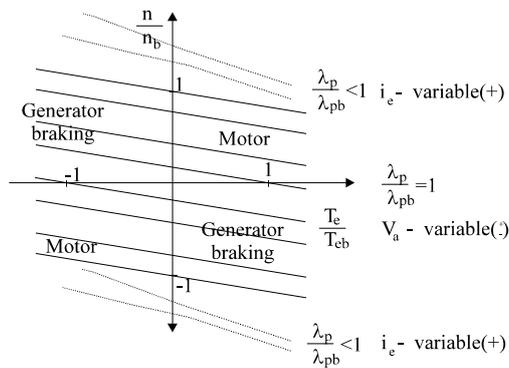
Figure 4.3. The torque/speed curves for variable speed
