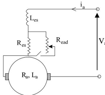
Figure 4.11. The DC brush series motor
