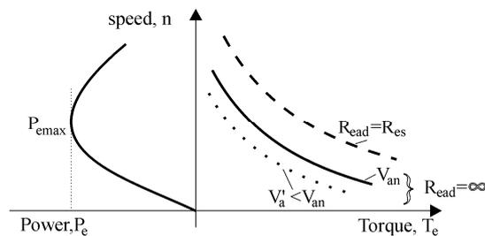
Figure 4.12. Speed/torque curve of DC brush series motor
