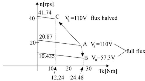
Figure 4.6. Torque/speed curves for varying speed from 1200 rpm (A) to 600 rpm (B) and, respectively, to 2400 rpm (C) for constant current.
