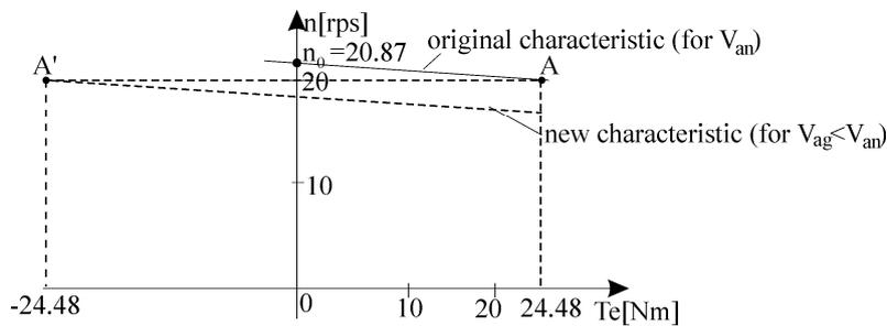
Figure 4.5. Torque/speed curves when switching from motoring to generating
