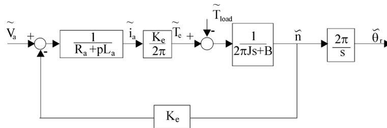
Figure 4.8. Constant flux block diagram of DC brush motor
