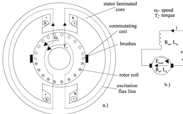
Figure 4.13. The two pole AC brush series motor
