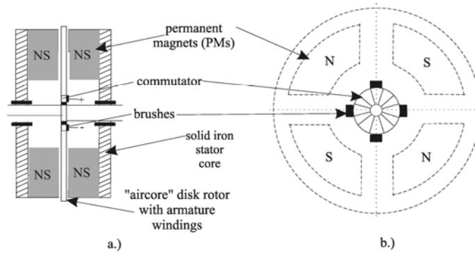
Figure 4.2. Disk DC brush motor ( $2p = 4$ poles)
