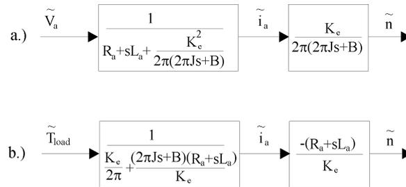
Figure 4.9. Cascaded transfer function for constant flux
