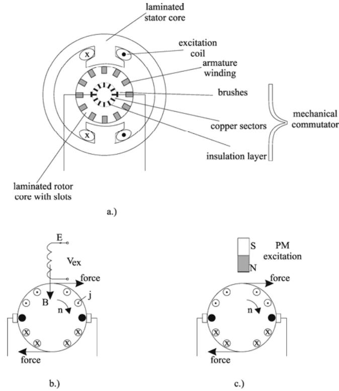
Figure 4.1. Cylindrical DC brush motor a.) topology, b.) schematics with electromagnetic excitation, c.) schematics with permanent magnets (PMs).
