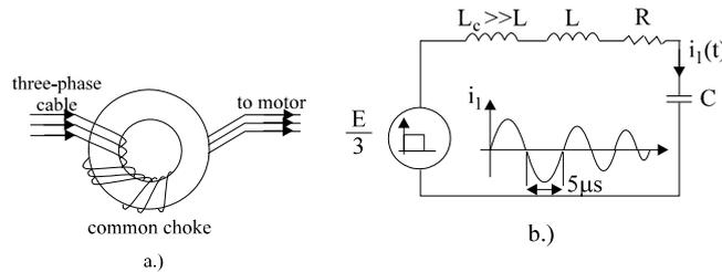
Figure 13.13. Common mode choke: a.) equivalent circuit, b.) leakage current  $i_l(t)$
