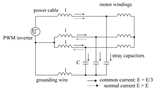
Figure 13.17. AC motor model with stray capacitors
