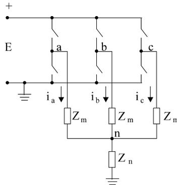
Figure 13.9. PWM inverter with motor and common mode impedance  $Z_n$  (isolated null point)
