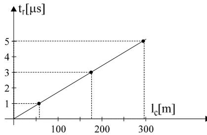
Figure 13.5. Voltage rising time  $t_r$  versus critical cable length
