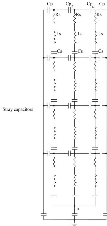
Figure 13.8. Motor RLC equivalent circuit for superhigh frequencies (stator only considered)
