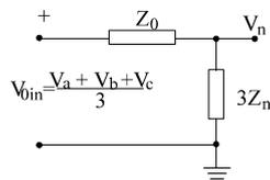
Figure 13.10. Motor model for common mode input voltage
