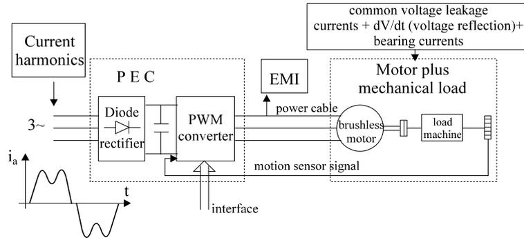
Figure 13.1. Basic PWM converter drive
