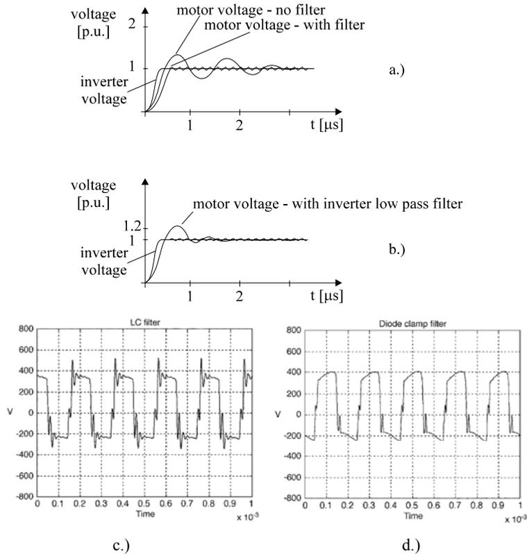
Figure 13.7. Motor terminal voltage: a.) with motor terminal RC filter, b.) with inverter low pass filter, c) 2.2 kW induction motor with low pass filter  $L_f = 2.6$  mH,  $C_f = 1.4$   $\mu$ F, d) 2.2 kW induction motor with low pass filter  $L_f = 2.6$  mH,  $C_f$
