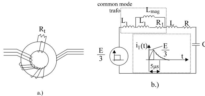
Figure 13.14. a.) common mode trafo, b.) equivalent circuit and leakage current response
