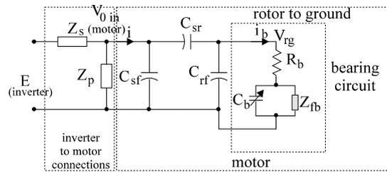
Figure 13.11. Common mode motor model for high frequencies
