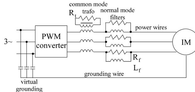
Figure 13.18. EMI reduction through common mode transformer and natural mode filters mounted at inverter output terminals
