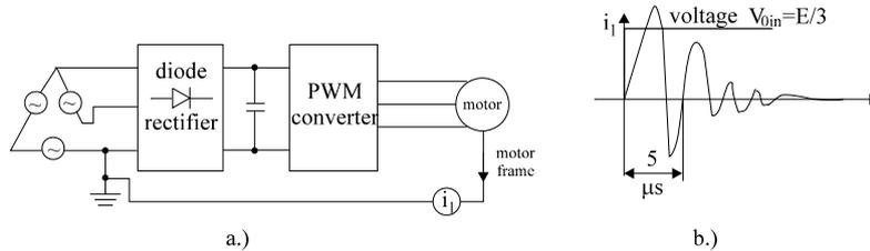
Figure 13.12. Measuring the leakage current: a.) test circuit, b.) current response to step voltage
