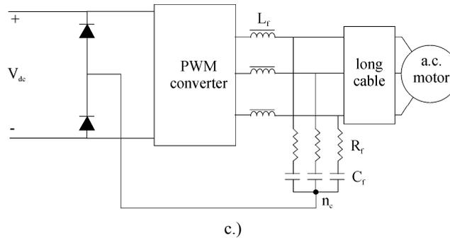
Figure 13.6. First-order filters: a.) at motor terminals, b.) at PWM converter output, c) LRC filter with diode clamp
