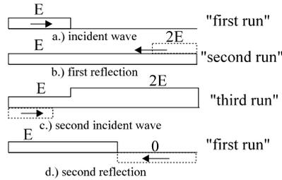
Figure 13.4. Reflection wave cycle
