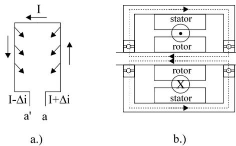
Figure 13.15. a.) current unbalance, b.) net flux and bearing circulating current
