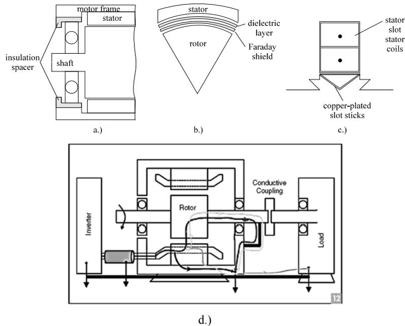
Figure 13.16. Methods to reduce bearing currents: a.) bearing insulation spacer, b.) conduction foil or paint, c.) conduction slot sticks, d.) one insulated and shaft grounding brush and motor, good high-frequency grounding from motor to load and from motor to drive
